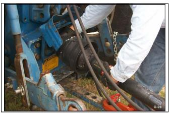
When attaching the Implement input driveline to the Tractor PTO, it is important that the **A WARNING** connecting yoke spring activated locking collar slides freely and the locking balls are seated securely in the groove on the Tractor PTO shaft. A driveline not attached correctly to the Tractor PTO shaft could come loose and result in personal injury and damage to the Implement. (S3PT-17)
